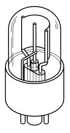
The curved surface of the cylinder is called the Cathode and is coated with a special compound that easily releases electrons when light (or photons) strike the curved surface. This coating is usually a ceasium (cesium in the USA) and antimony alloy on silver oxide.
