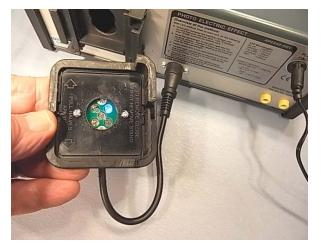
This image shows the 5 LEDs grouped tightly to provide good cathode illumination in the photo-cell. A switch selects each LED colour and the brightness or intensity of any colour can be adjusted by the 'intensity' control on the front panel. The photo-cell itself can be seen through the orifice in the rear of the instrument however it is always best to keep the orifice covered by the LED panel so the photo-cell is always in total darkness.
