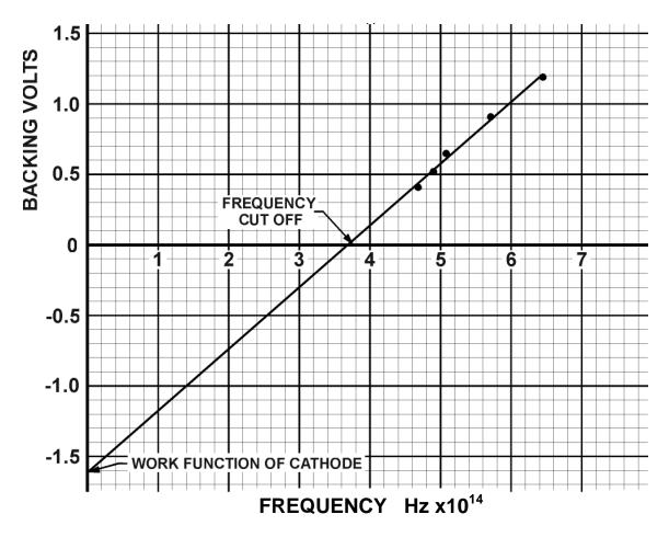
Slope of graph =  $\Delta V / \Delta f$  = 1.50 / 3.77 x 10<sup>14</sup> = 0.39 x 10<sup>-14</sup> = h/e
