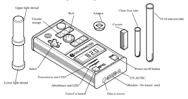
The front panel provides a large LCD digital display and two press buttons. Right hand button is power ON/OFF and the left hand button is for changing the desired unit from 'Transmission' to 'Absorbance' and a longer press performs the zero and 100% 'Calibration' of Transmission and 0 to 2.3 of Absorbance. A mini LED indicates which Unit is selected.
