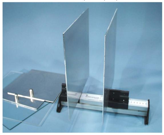
Physical size: 200x200mm plates, 283x283mm plates, 0-160mm gap. Weight: 3.1 kg Glass and acrylic dielectric: 290x290mm x3mm thick
