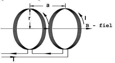
THE MAGNETIC FIELD CREATED BY HELMHOLTZ COILS:
