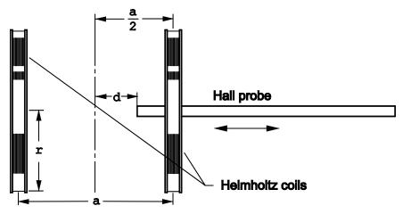
a = separation of coils r = mean radius of coils d = distance of the Hall device from the mid point between the two coils.
