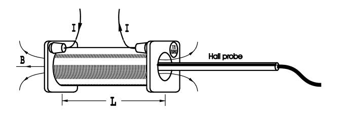
Select meter to read amps and adjust the current through the solenoid to 1.7 amp. Use the equation " $B = \mu_0 nI$  newtons / amp-metre "to calculate the expected field strength. The number of turns in the solenoid is marked on the coil. To find **'n'** number of turns per metre length of solenoid winding, **divide number of turns in the coil by length of coil in metres.**
