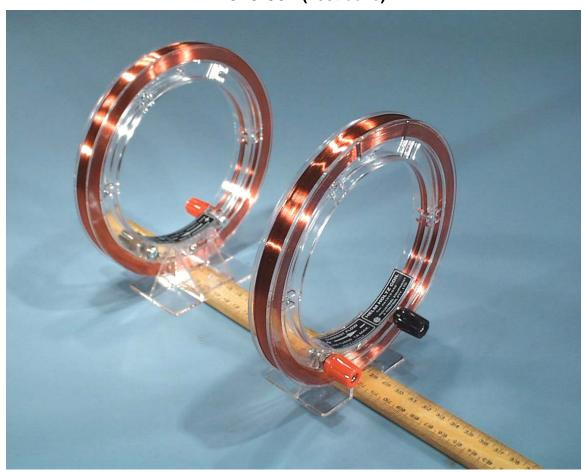
Physical size: 115mm ID 163mm OD 150mm average winding diam. 400 turns
