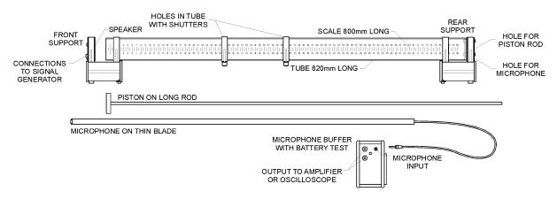
**HOW IT WORKS:** Look at the drawing above to see the various parts of the Kundt's Apparatus. Variable length air column with loud speaker to create the sound waves and miniature microphone to detect the nodes and antinodes inside the tube.
