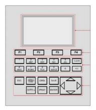
Stand-alone model has built-in software for full functions, thus eliminating the need for optional Windows analysis software (with a protection dongle) to control the spectrophotometer via a PC
