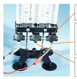
If platinum electrodes are to be stored, they are easily removed by hand from under each tube.
