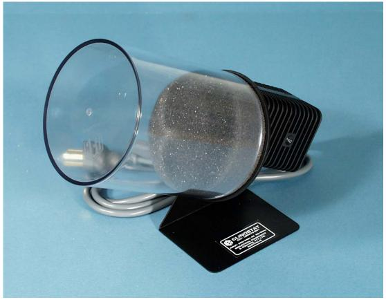
Physical size: 250x110mm LxD Weight: 1.0 kg approx. 4 revs/hour
