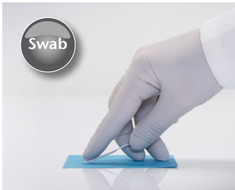
Figure 1: RIDA®QUICK Gliadin dip stick can be used directly as a swab test
